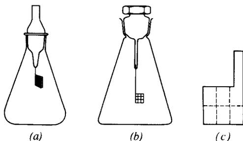
Fig. 3.11 Conventional flasks for microdeterminations: (a) air leak design; (b) stopper design; (c) filter paper for wrapping sample. Reproduced by permission from A. M. B. Macdonald, in *Advances in Analytical Chemistry and Instrumentation*, C. N. Reilly (Ed.), Vol. 4, Interscience, New York, 1965, p. 75.
