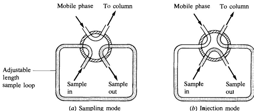
**Fig. 8.3 Operation of a sample loop.**
