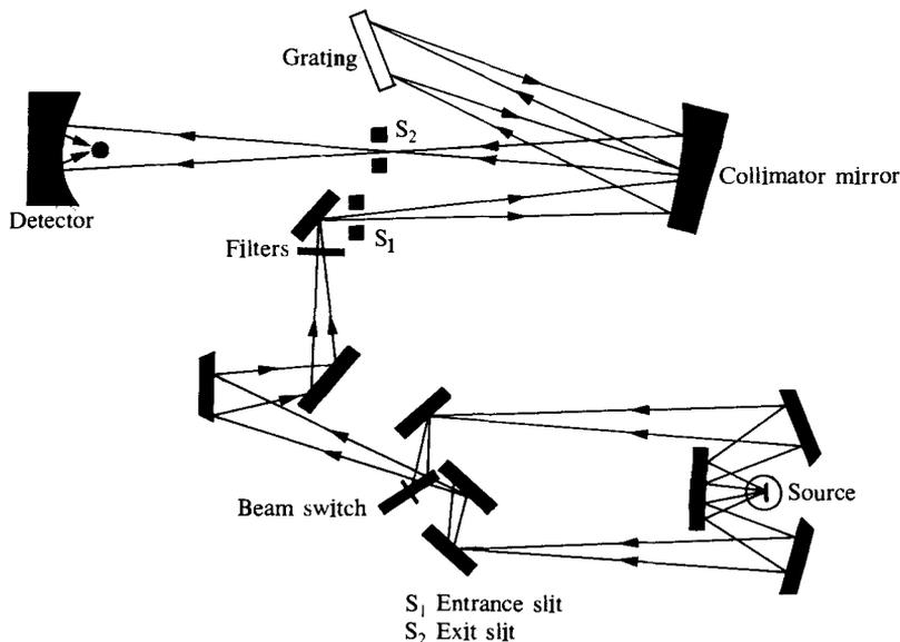
**Fig. 19.2** Layout of an infrared spectrophotometer employing a diffraction grating for monochromation. Reproduced by permission from R. C. J. Osland, *Principles and Practices of Infrared Spectroscopy*, 2nd edn, Phillips Ltd, 1985.
