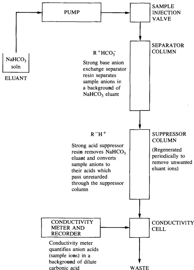
Fig. 7.3 Ion chromatography flow scheme (anion analysis).
