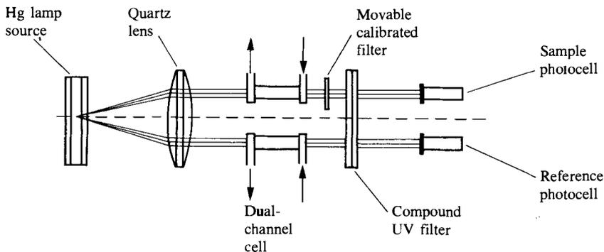
Fig. 8.5 Block diagram of a double-beam UV detector.
