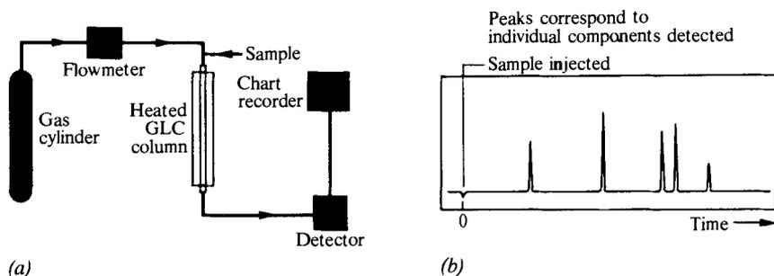
Fig. 9.1 (a) Block diagram of a gas chromatograph. (b) Typical chart record. Reproduced by permission from R. C. Denney, *The Truth about Breath Tests*, Nelson, London, 1970.
