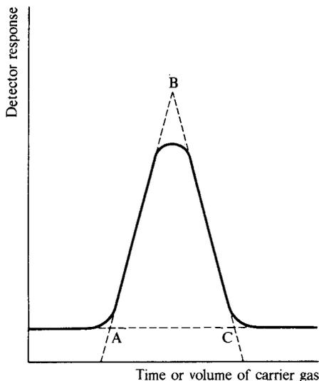
Fig. 9.3 Measurement of peak area by triangulation.
