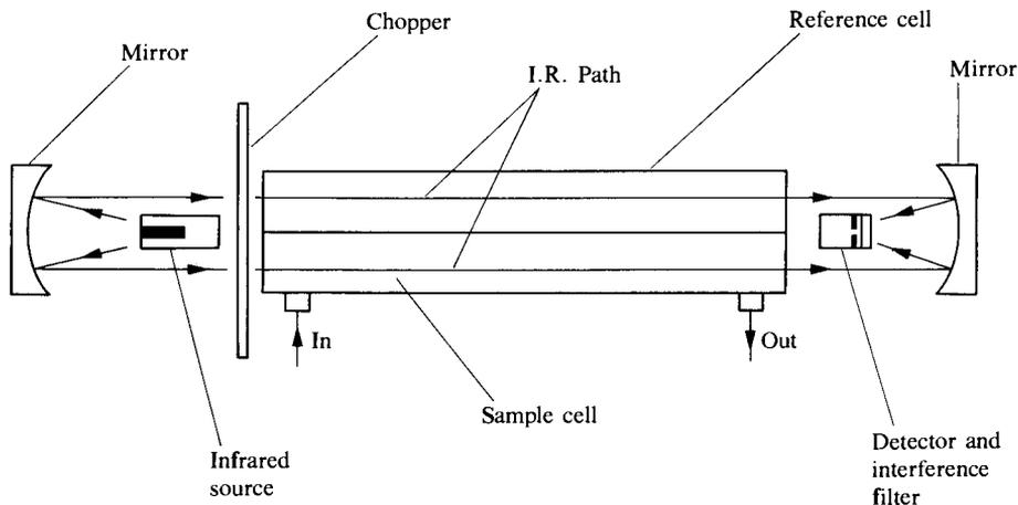
**Fig. 19.5** Diagram of the infrared analyser unit of the Lion Intoximeter 3000 breath alcohol analyser. Reproduced by permission of Lion Laboratories Ltd, Ty Verlon Industrial Estate, Barry, Wales CF6 3BE, UK.
