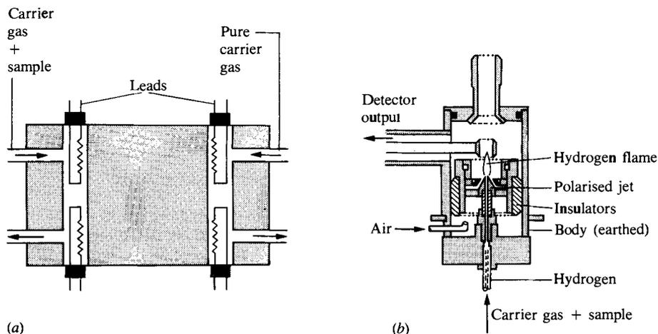
Fig. 9.2 (a) Thermal conductivity detector. (b) Flame ionisation detector.
